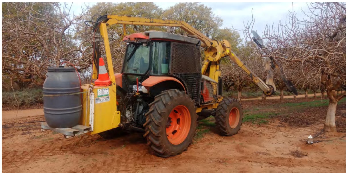
The 4 bladed hedging/tipping/topping/skirting machine.
